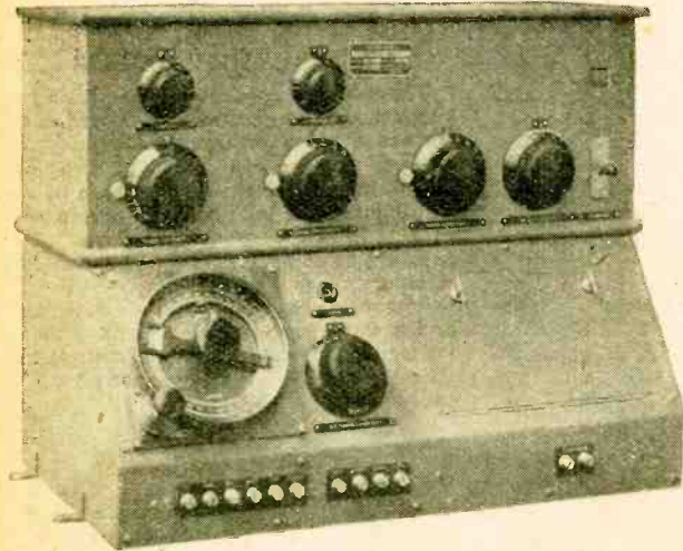
The new Marconi direction finder, with screened grid H.F. amplifying valves and semi-ganged tuning.
